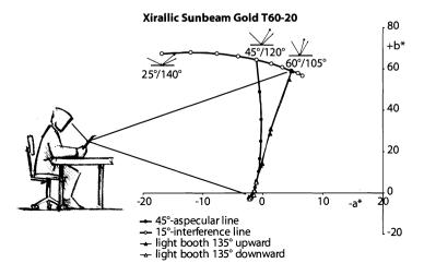
+20°. The viewing angle will change from 70° to 60°, the angle of specular reflection will become 120° and the viewing angle will become 100°. No such angular relationships are implemented in any items of photometric instrumentation.
