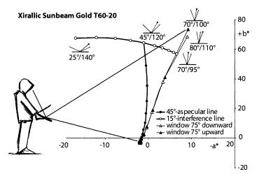
reflection will then change from  $100^{\circ}$  to  $95^{\circ}$  and  $90^{\circ}$ , respectively; the viewing angle will change from  $110^{\circ}$  to  $115^{\circ}$  and  $120^{\circ}$ , respectively, and their difference will change from  $-10^{\circ}$  to  $-20^{\circ}$  and  $-30^{\circ}$ , respectively (Figure 4).
